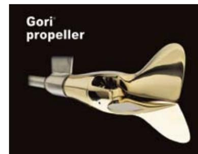
A well known name in folding props, the two-bladed Gori folding propeller is for sailing yachts fitted with engines up to 60hp and is available in seven diameters for shaft and Saildrive installation. The geared design ensures blades open and close together, giving less vibration under way, with the blades closing simultaneously when sailing.
