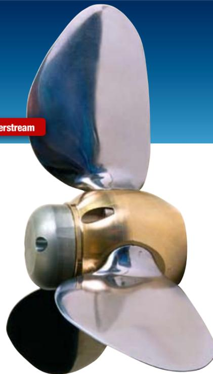
Volvo Penta folding propellers are made from a highly corrosion resistant, nickel-aluminium-bronze alloy and, because the blades and hub are sold separately, you can easily put together a match to meet the specific needs of your yacht.
